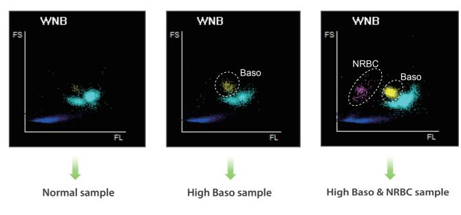
BC-6200 provides accurate results on samples even with high level of Basophils and NRBCs.
