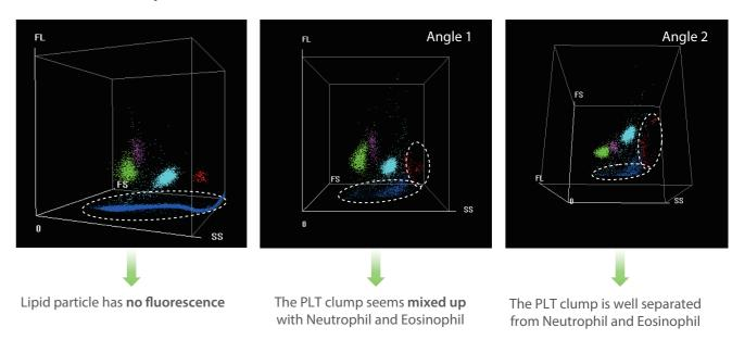
In DIFF scattergram, WBCs are dyed, but not lipid particles, by fluorescence, which prevents interference and ensures more accurate WBC results.
